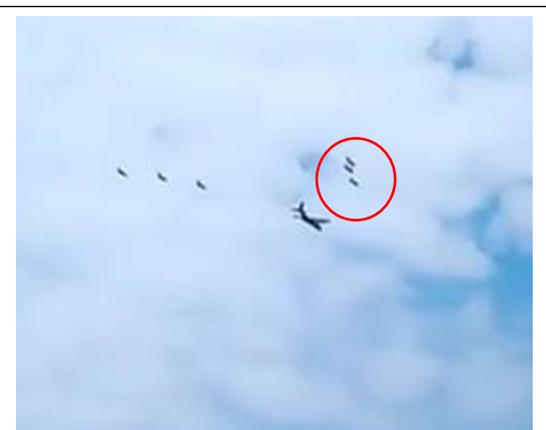
The right-hand VIC No.3 was lagging and during the acceleration to station, left no lateral separation for the join up resulting in a wing to wing collision.
